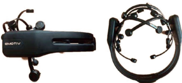
Figure 1. Wireless helmet Emotiv Epoc
