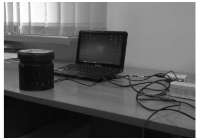
Figure 2. Testing station for assessment of reproduction of hand pressure force – dynamometer
