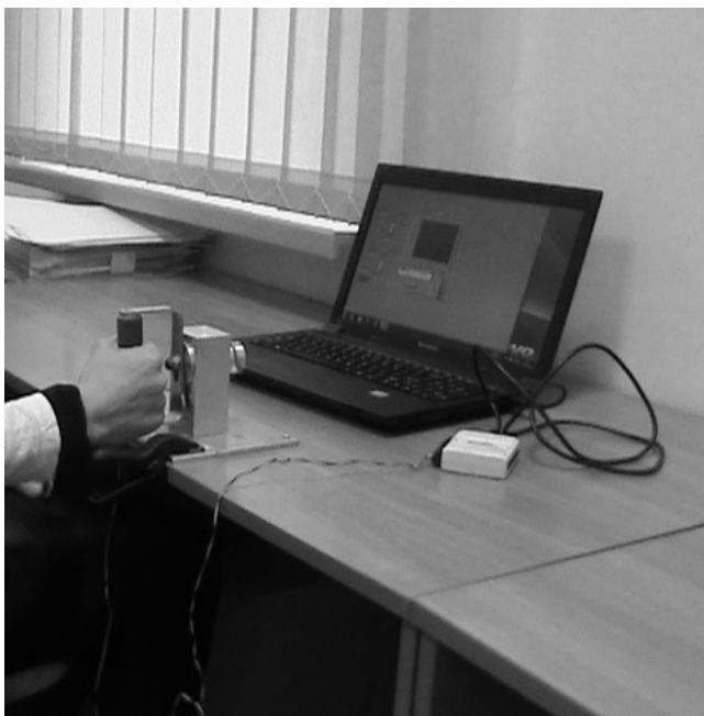
Figure 1. Testing station for range of movement assessment – goniometer
