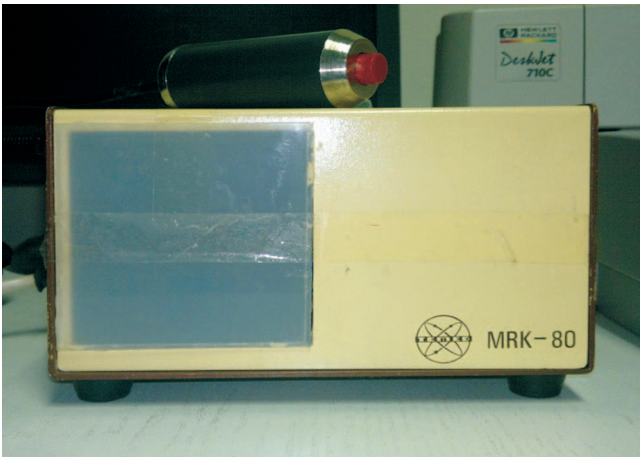
Figure 1. The screen for emission of visual stimuli with the manual reaction button
