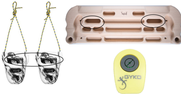
Figure 1. Portable holds (left), fingerboard (upper, right), and Gyko inertial sensor (bottom, right). The ovals mark the holds on which the subjects performed pull-ups
