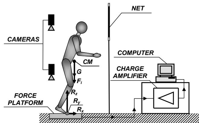
**Figure 1.** Biomechanical model during landing in volleyball jump ( $R_z$  – the vertical component of GRF,  $R_y$  – the anterior-posterior of the horizontal component of GRF,  $R_x$  – the lateral of the horizontal component of GRF,  $G$  – gravitational force,  $F_i$  – inertial force,  $CM$  – center of mass)
