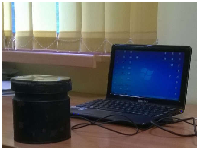
Figure 2. Testing station for assessment of hand pressure force reproduction – dynamometer
