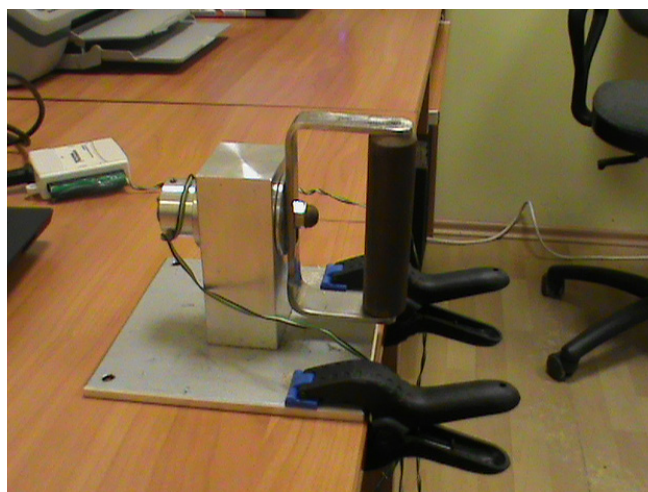
Figure 1. Testing station for assessment of the range of motion – goniometer
